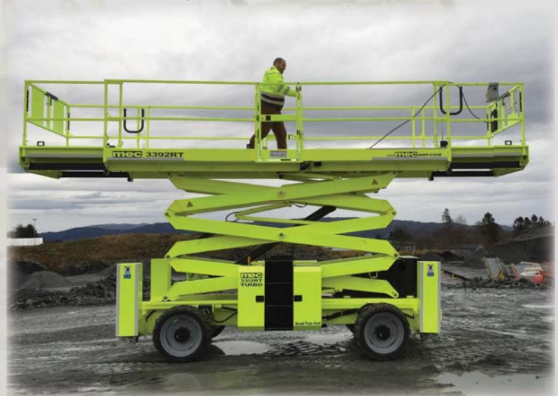
7.54m platform with Dual Decks extended
